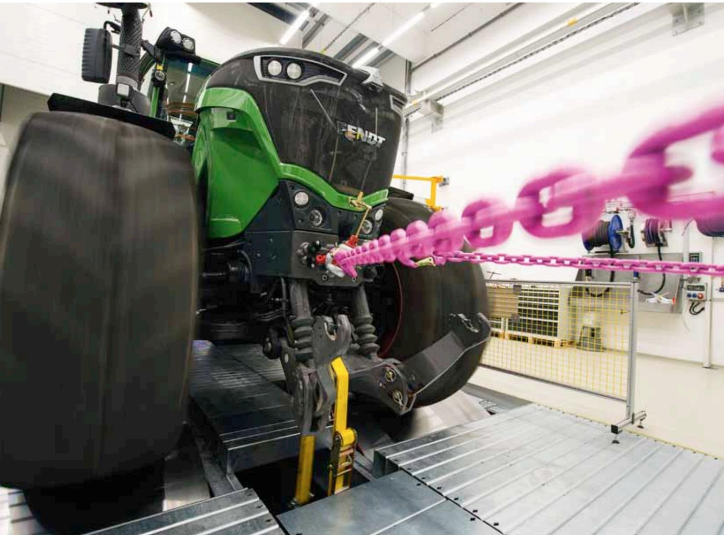
The standardised pink chains can withstand forces of up to 20 tonnes.
