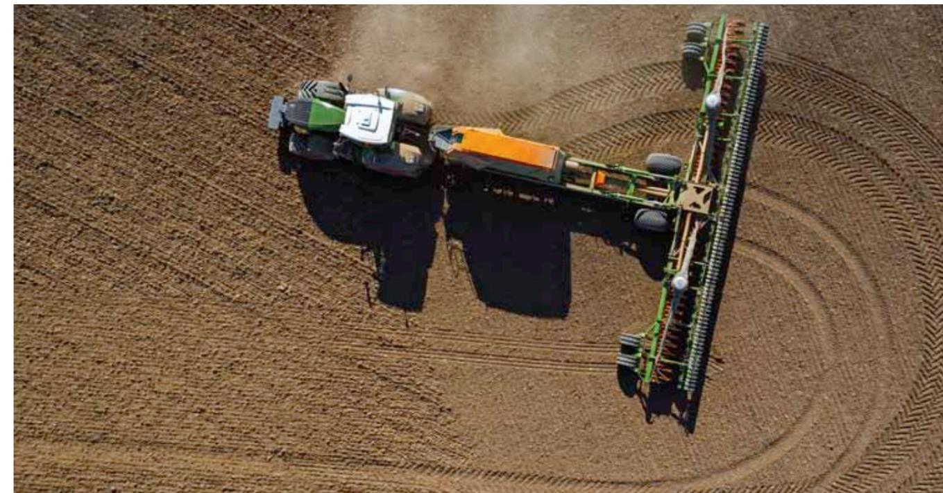
“Pull-in-turn” effect: Thanks to the variable four-wheel drive, the front wheel pulls the tractor into the curve and reduces the turning circle by an additional ten percent or 1 metre.
