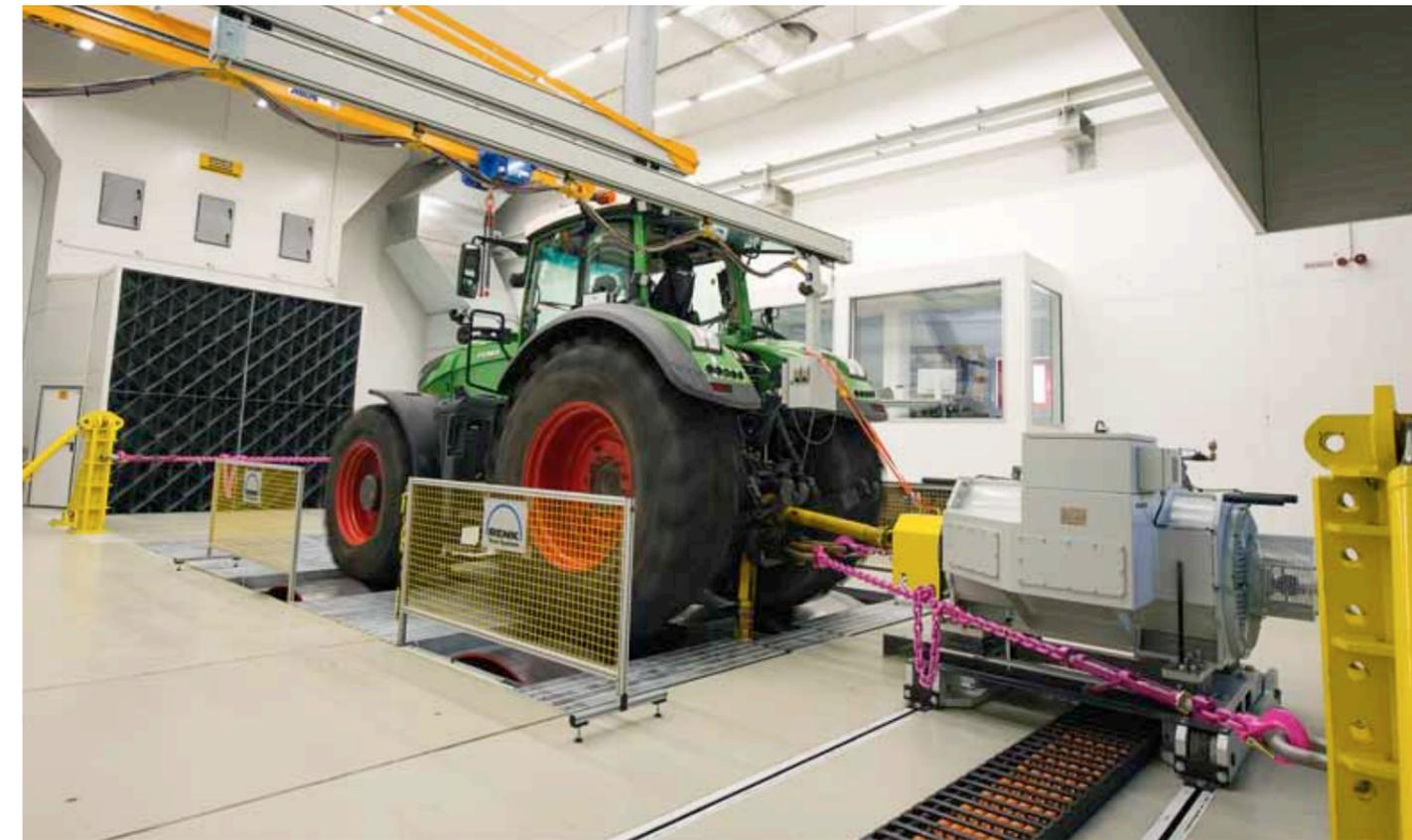
In the background: The honeycomb-shaped supply nozzle blows air into the testing room, creating laminar (without turbulences) flow of up to 20 km/h.
