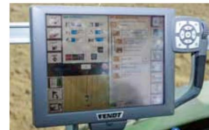
Fendt Terminal, VarioDoc, main page: The field to be worked and the waylines can be clearly recognised in the lower quarter of the terminal. The machine, operator, field, type of crop and the operation are documented on the right side in the main menu. After the work has been completed, the data are sent to the office computer.
