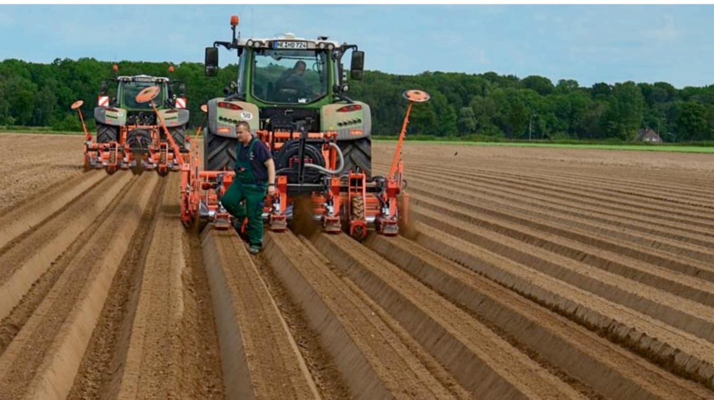
The machine combinations each pull four dams with carrot seeds precisely with VarioGuide RTK.
