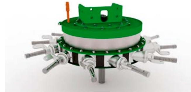
The rotor is integrated in the existing housing of the rake socket as an external rotor.
