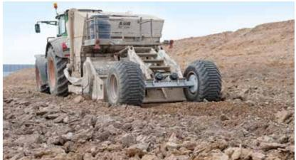
Fendt 930 Vario with a SBF 24-6 soil stabiliser. The mixed binder is determined according to the soil type as well as the moisture class, e.g. B50 is 50% lime and 50% cement (Foto: Daniela Müller)
