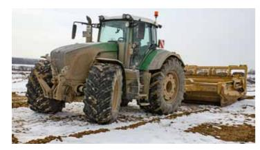
Earth is removed with a scraper bucket to reach the underlying layer of sand.
