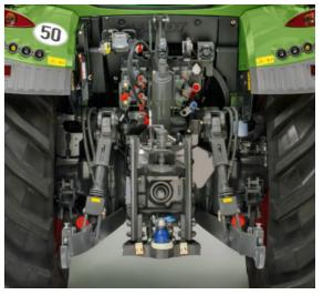
■ In the Fendt Vario tailgate, there are interfaces for the mounting of various implements, e.g. hydraulic connections, PTO or trailer system. The main feature of the tailgate is excellent visibility and accessibility.
