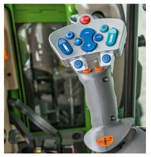
■ The 200 V/F/P Vario includes additional control valve functions and automated functions for the rear linkage and rear PTO, which can be controlled with the multifunction joystick. TMS comes integrated as standard, and allows up to six control units.
