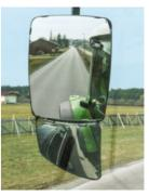
■ The wide-angle mirror expands the field of vision, which greatly enhances safety. You have a better overview of things, especially what is happening on the sides of the tractor. The hazard zone, which is usually located in the blind spot, is more clearly visible.
