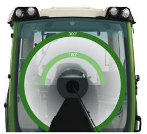
□ The 300° wiper offers a completely clear view. To keep the view onto the wheel arches and the front implement clear, the wiper field is almost doubled – with an integrated interval switch.
