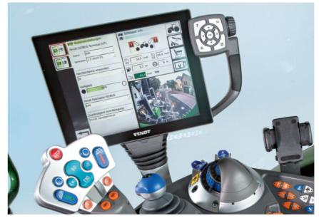
The Varioterminal 10.4" offers various display options. The operator can display up to four applications on the terminal. The camera view proves especially practical: Up to two rear view cameras in half-frame view or a camera in full frame offer a good overview and therefore increased safety.
