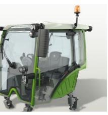
Fendt offers a sophisticated suspension concept for all series. The Fendt 200 and 300 Vario series can be equipped with a cab suspension on request, with the cab suspension being standard from the 500 Vario series onward. Pictured: The four-point comfort cab suspension with integral self-levelling reduces vibrations
