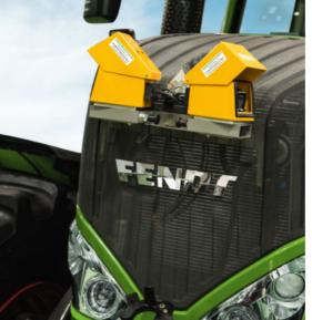
□ The front camera system allows you to safely ride with implements that protrude towards the front, even on the roads.
