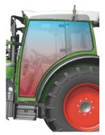
□ The optional floor heater is ideal for use in winter. Controlled by temperature sensors, the footwell is heated quickly and efficiently.
