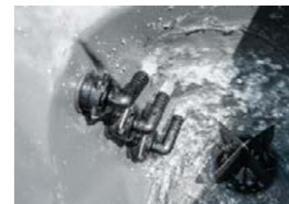
High-performance diffusers on the internal wall and in the overflow optimise the rinsing process.
