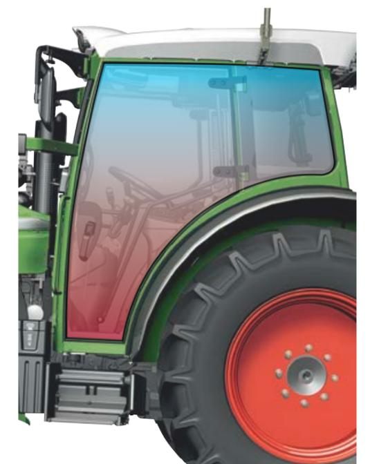
▲ Schematic temperature distribution in the cab. Cooler temperature in the top section, warmer temperature in the lower section.
