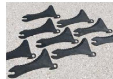
The elongated knives with serrations on one edge ensure an efficient, pulling cut, and can be removed without the use of tools.
