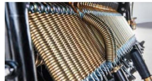
Each knife is fully protected with the Trimatic foreign-body guard system, also available on the Fendt Tigo ST, S and MS.
