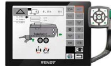
Control the bulkhead and the table of the Tigo MR Profi directly via your terminal. Even the pick-up and drawbar can be conveniently adjusted from here.
