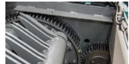
The swing-arm unit is powered with low-wear gears with extra strong spur gears.
