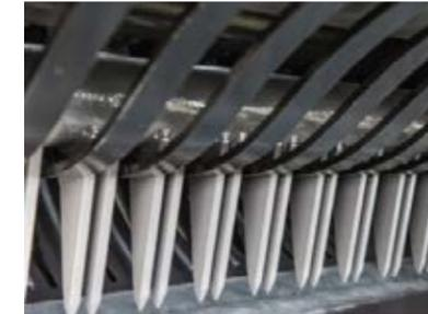
The single-section conveyor swing arm allows an even and smooth forage flow.
