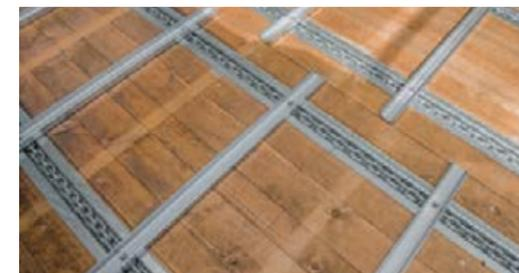
With the four 10 mm thick round steel chains of the large Tigo MS, MR and all MR Profi models, with 50 t breaking load you are prepared for even the toughest applications. The small Tigo MS and MR models provide support with two scraper floor chains and 25 t breaking load. You can also opt to equip the smaller models with four chains and offset scraper bars.
