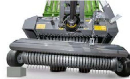
The trailing gauge wheels of the automated pick-up release it on corners, can be turned and thus protect the sward. Adjust the height of the wheels with a series of holes.
