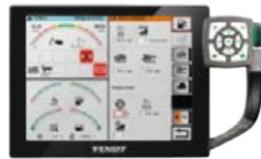
The engine load reduction and maximum driving speed with the automatic maximum output control can be set in the terminal in order to adjust the automated function to the prevailing conditions.
