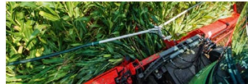
The maize header is available with eight, ten or twelve rows. For on-road driving, the header folds up hydraulically, so it can be brought into transport position quickly.
