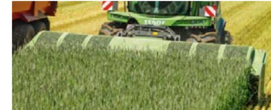
The sturdy whole crop header is designed for deep, loss-free cuts in different kinds of crops. When harvesting biomass, it delivers the best silage with a minimum of contamination.
