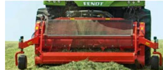
The Pickup P3003 Maximum with HD drive achieves high output even under extreme harvesting conditions. The centrally integrated feeler wheel ensures better ground following.
