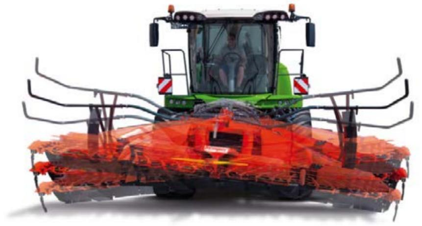
Together with the innovative swinging frame directly on the intake, ground-contact sensors actively adapt the header to the ground contour.
