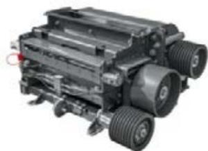
To prepare the crop even more intensively, you can order via AGCO Parts a cracker drive with a 40% instead of a 30% speed difference between the two cracker rollers.
