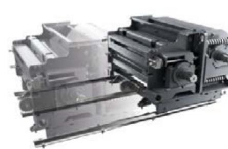
No grain gets past the ultra efficient R cracker with sawtooth profile. Thanks to the vast processing space between the large rollers and a speed difference of 30% or 40% between the two conditioner rollers, it delivers superior pulping results.
