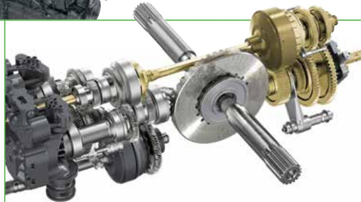
Stepless Vario CVT, with no clutch packs, optimizes engine power and fuel economy, with seamless travel from 61 ft/h to 31 mph
