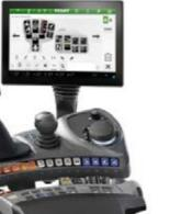
Power Setting 2 - Crossgate lever - No rocker pair (linear module) to control the hydraulic valves
