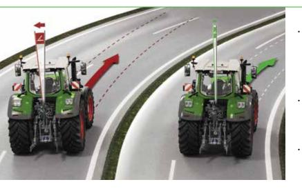
Optional Fendt Stability Control (FSC) takes steering precision, driving stability and braking safety to new levels. At speeds above 12.4 mph (20 km/h), FSC locks the front axle suspension cylinders and dampens side-to-side movement to ensure maximum stability in transport. When speeds drop below the FSC threshold, it automatically disengages to ensure maximum ground contact with all four tires
