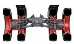
VarioGrip<sup>™</sup>, our factory-installed tire inflation and deflation system allows the operator to set and control tire pressure, ensuring minimal compaction, less tire wear, and maximum performance in the field or on the road
