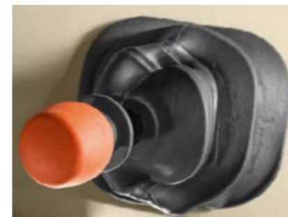
Hand brake assistant in automatic position: The hand brake is automatically activated.
