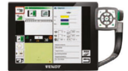
The Varioterminal informs you about the next maintenance and servicing dates, it even has a reminder function.
