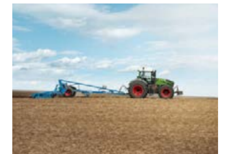
Thanks to the TMS tractor management system and the automatic maximum load control 2.0, the tractor adapts the engine speed optimally to the road speed.
