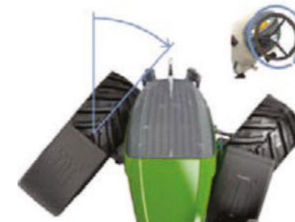
With VarioActive, you already go through the full steering angle with just one turn of the steering wheel.
