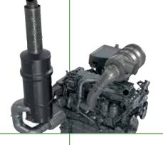
The powerful six-cylinder engine maximizes efficiency through its Tractor Management System (TMS); set the desired speed, activate the TMS and the system automatically adjusts for optimum performance
