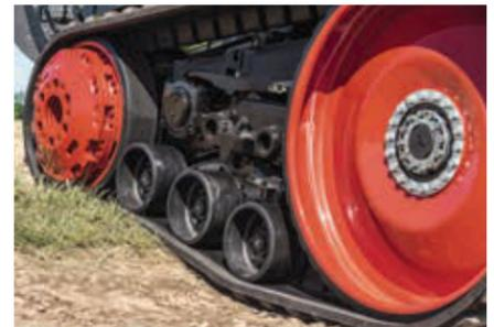
Our patented Mobil-Trac System (MTS) provides an operator with better traction, and with reduced compaction, thanks to its long footprint and pivoting midwheel design. Paired with our Smart Ride and cab suspension system, it provides exceptional ride quality down the road or through the field.
