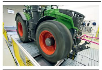
Top photo: The standardized pink chains can withstand forces of up to 22 tons. Above: The distance between the axles can be flexibly adjusted from  $6\frac{1}{2} - 19\frac{1}{2}$  ft, which ensures that all tractors can be tested – from the 200 Series to the 1000 Series.
