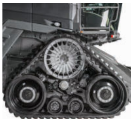
The TrakRide crawler drive minimises ground pressure.
