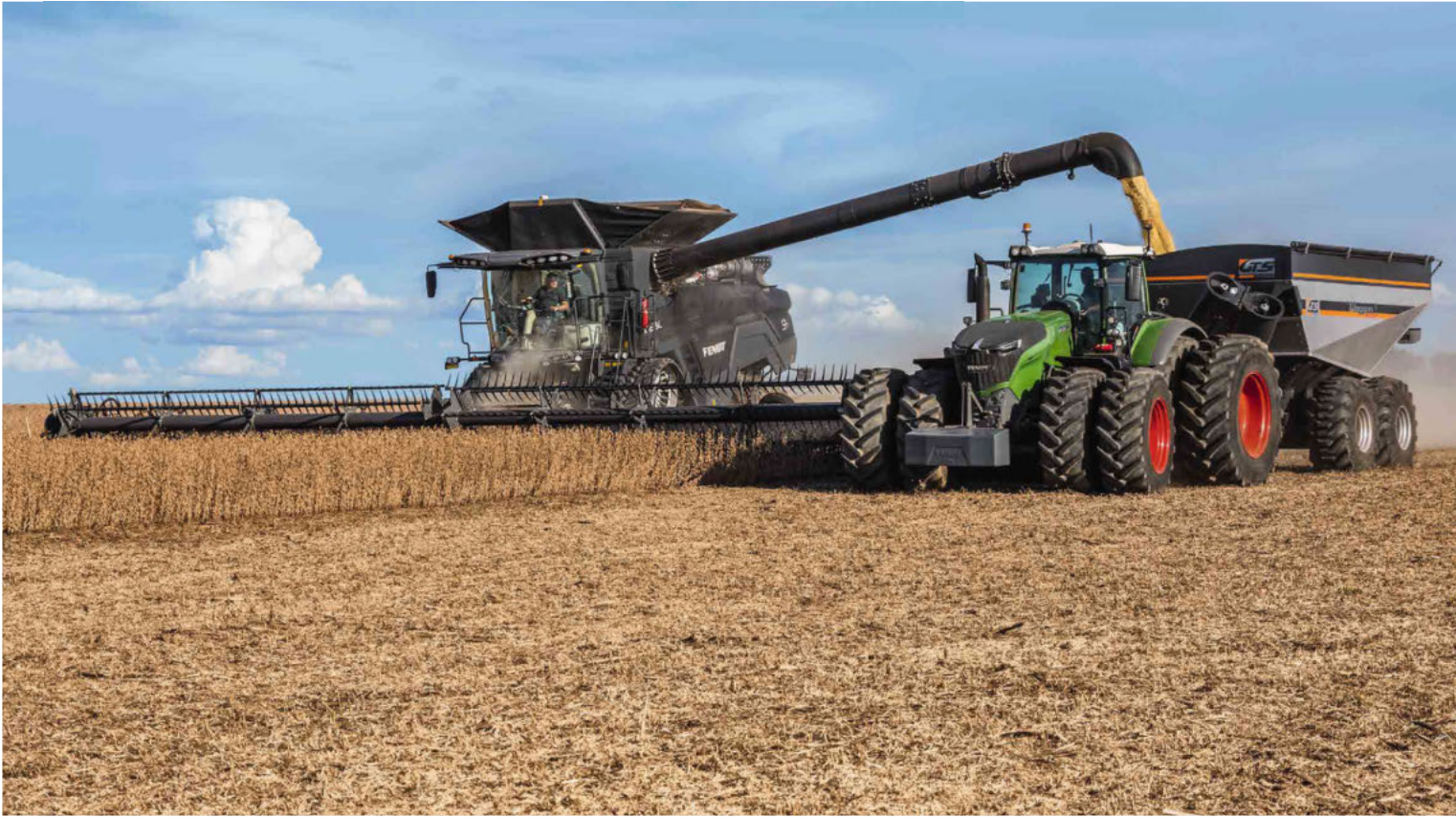
Fewer and shorter stops for unloading are soon reflected in a greater daily yield – sensors for yield and moisture and a grain quality camera are fitted to the elevator. The data is accurate to 98%, and applied with the VarioDoc ISOBUS standard, live yield mapping and IDEALharvest™.
