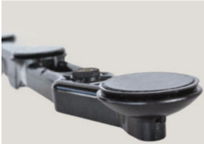
Loss sensors at the end of the shaker shoe help the operator adjust the machine to the best possible configuration, by recording crop which falls to the ground via pressure and acoustics.
