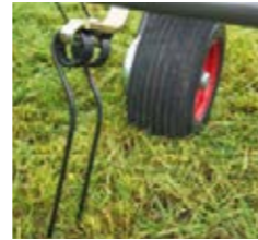
The 'Super C' tines are made from 9.5 thick heavy-duty steel, and are marked for their long service life and exceptional results.
