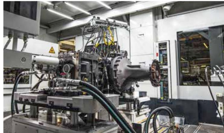
Undergoing thorough testing: a Vario transmission in the enclosed testing booth. Afterwards only 100 percent quality is built into the tractor.
