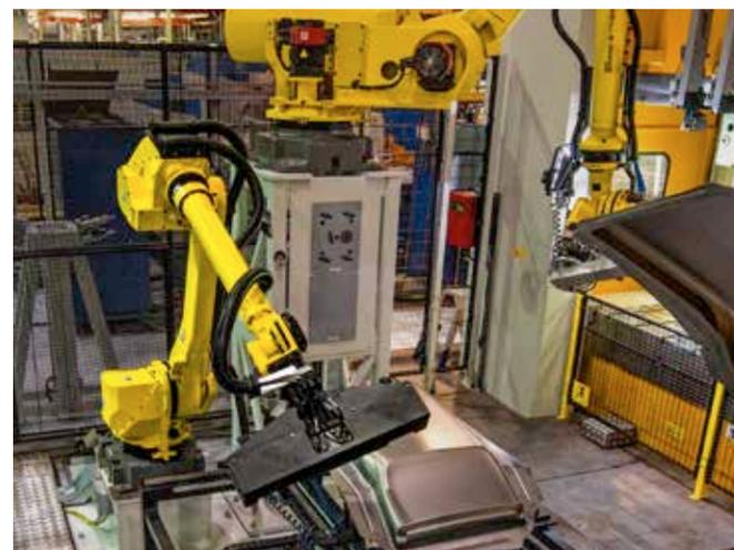
A laser scanner tests the surface of a tractor bonnet after deep drawing in the press
