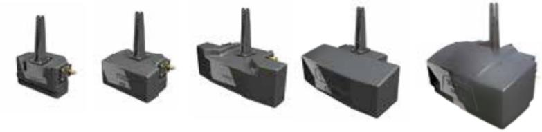
Ballasting options: Fendt offers you up to 24 different combinations of front and wheel weights. Fendt solutions are just as versatile as your tasks.
