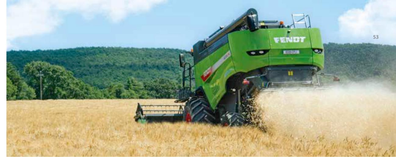
Enhanced performance through the PowerFlow table with up to 7.70 cutting width.
