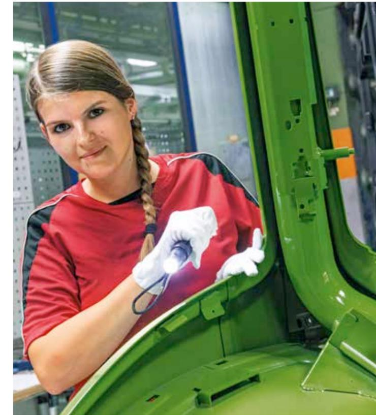
Cab quality control: After the tractor cab comes from the painting facility, the staff checks the quality of the coat of paint.
