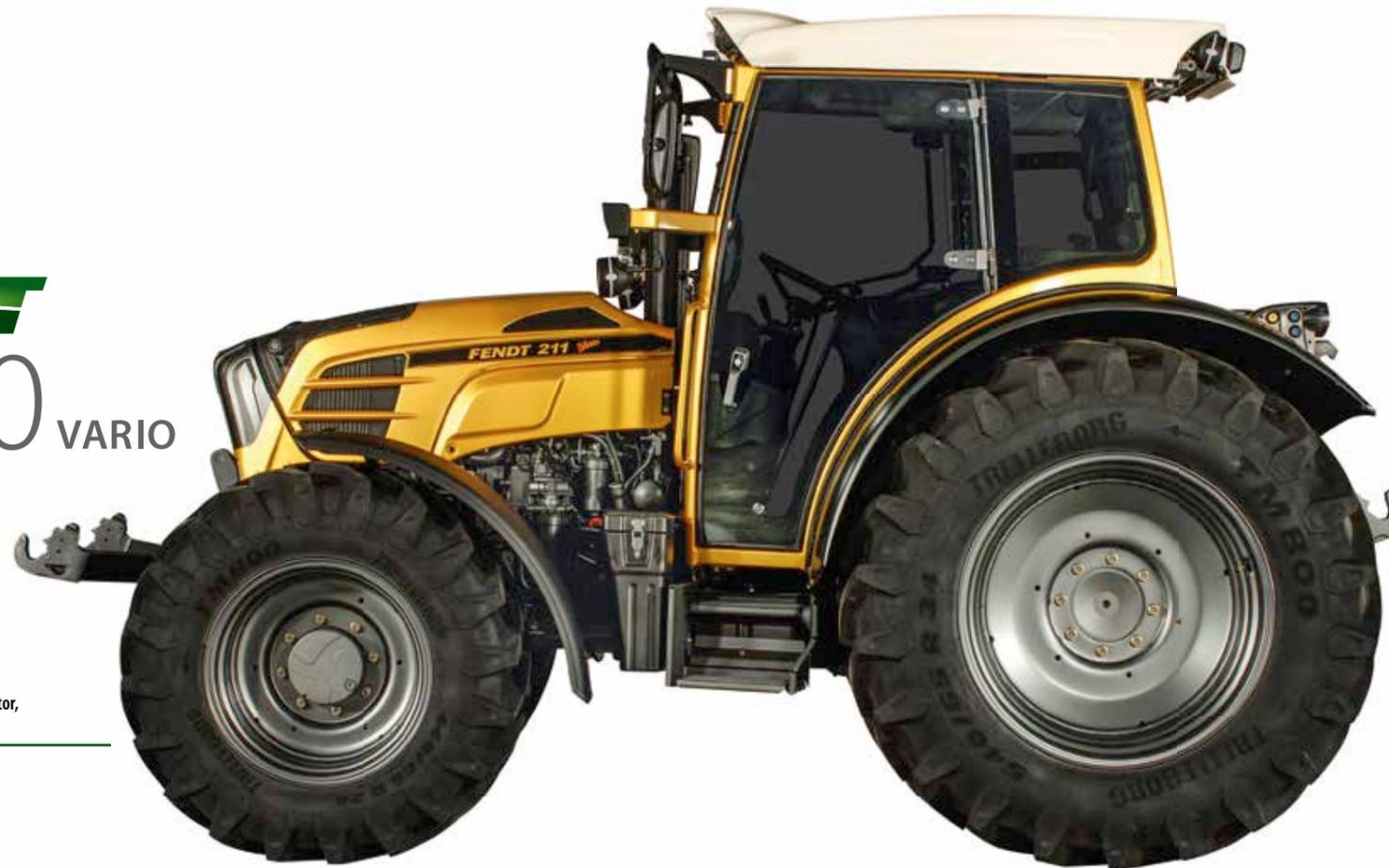
The 100,000th Vario transmission is the heart of this gold Fendt 211 Vario, built in 2009. Since then, every Fendt tractor, from the largest to the smallest, is stepless.
